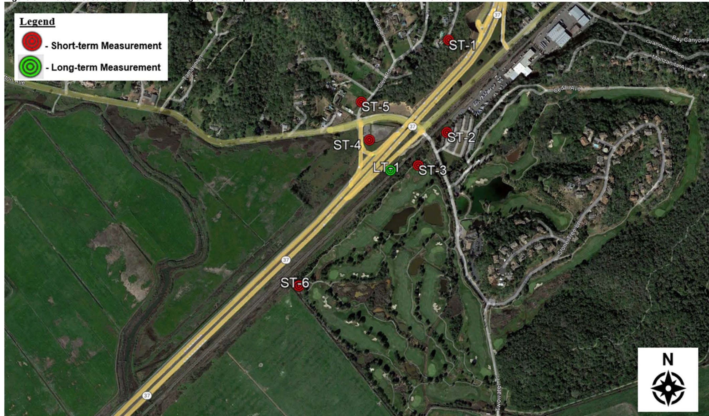
Figure 5-1. Noise Measurement Positions along the eastern portion of the SR 37 corridor, near Atherton Avenue
