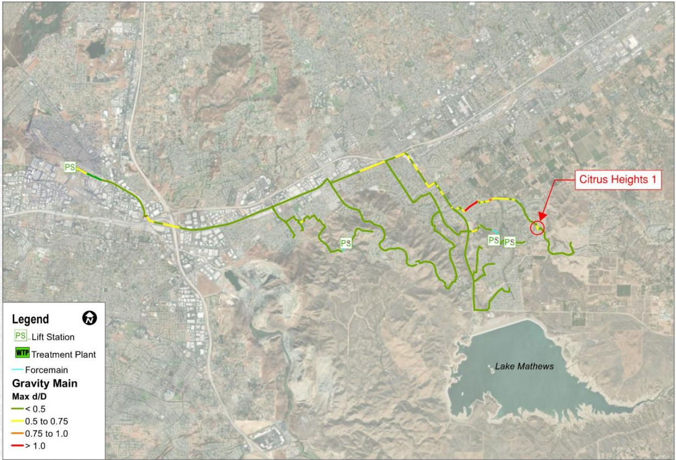
Figure 8-3: Near-Term Sewer Gravity and Force Main Recommendations 1
