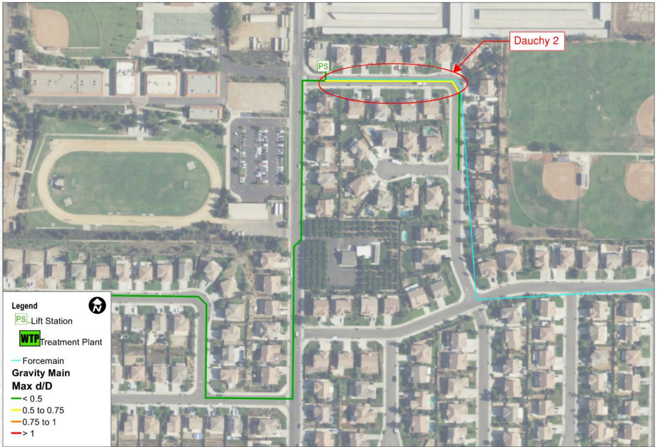
Figure 8-6: Ultimate Sewer Gravity and Force Main Recommendations 2
