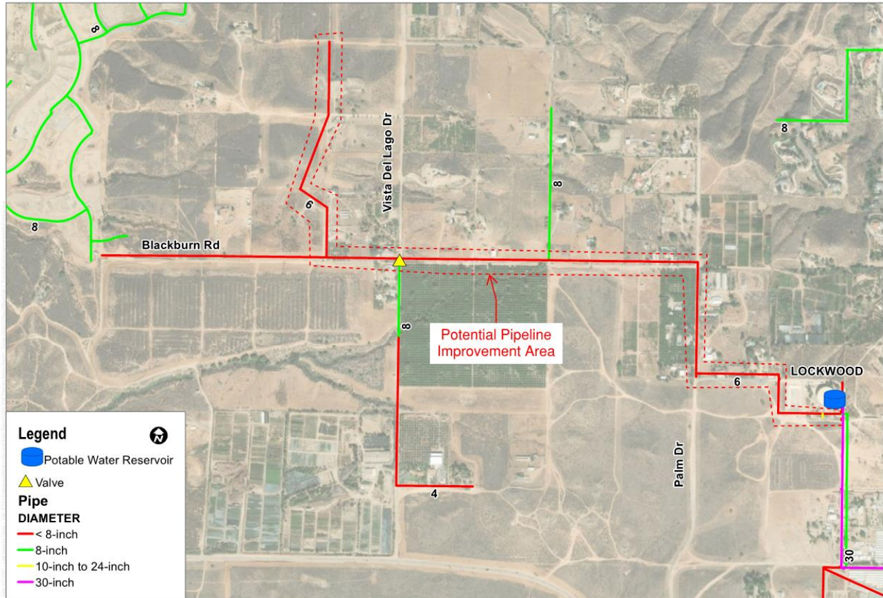
Figure 6-4: CIP W-2 Potential Pipeline Improvements - Blackburn Road
