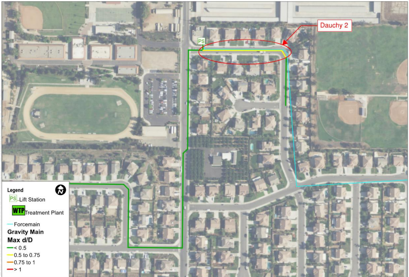
Figure 8-6: Ultimate Sewer Gravity and Force Main Recommendations 2
