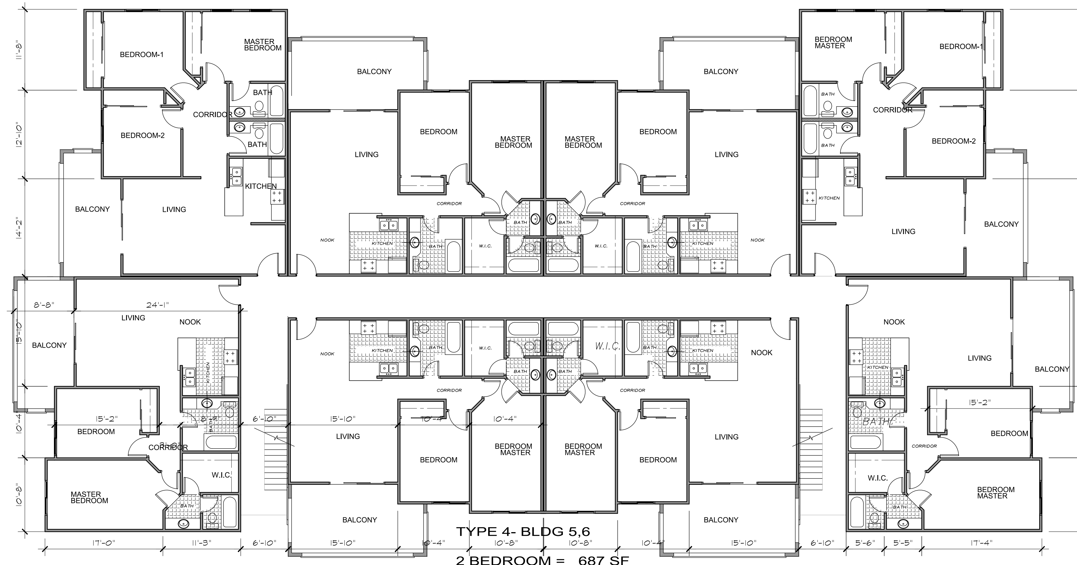
1ST & 2ND FLOOR PLAN - TYPE 4 SCALE 1/8" = 1'-0" TYPE 4- BLDG 5,6 2 BEDROOM = 687 SF 2 BEDROOM = 962 SF 3 BEDROOM = 1,027 SF
