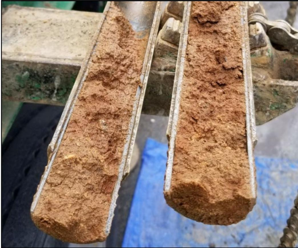
Figure 4-3. Unit 2 Older Alluvium (Qoa)
