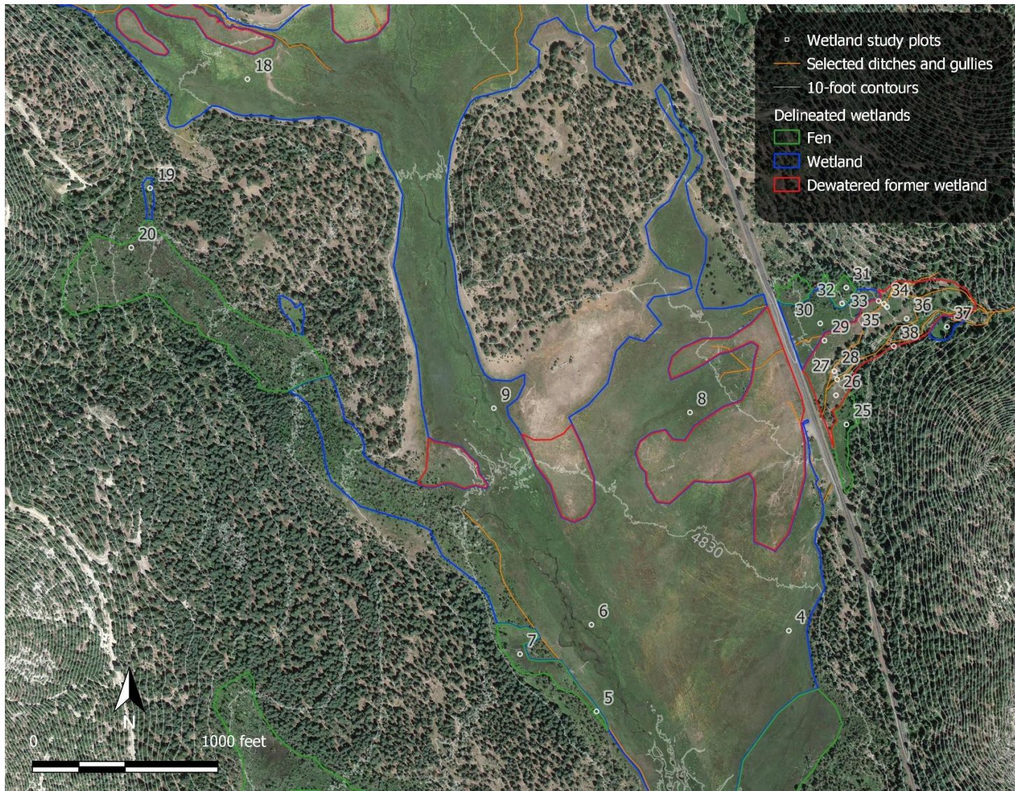
Figure 6. Zoom in on the third from top section of Childs Meadow. Plot 20 is a treed fen, plots 25-37 cover a range from intact fens to deeply gullied and dewatered wetlands. A long ditch runs from north of plot 7 south of plot 5, intercepting groundwater discharge the plot 20 and plot 7 fens and conveying it rapidly downstream.
