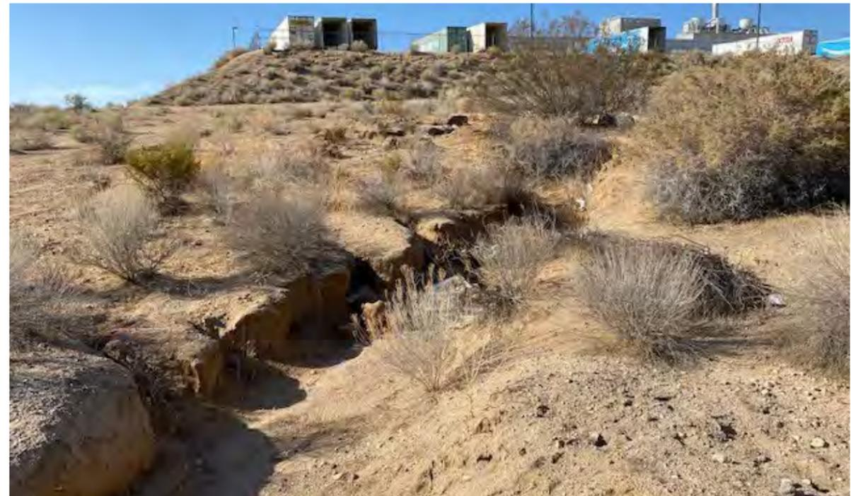
Photograph 8: Photo looking southwest and upstream at Drainage C from the eastern perimeter of the Project site. Photo depicts incised nature of Drainage C.
