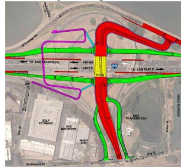
Alternative 2: Single Point Diamond with T-Intersection
