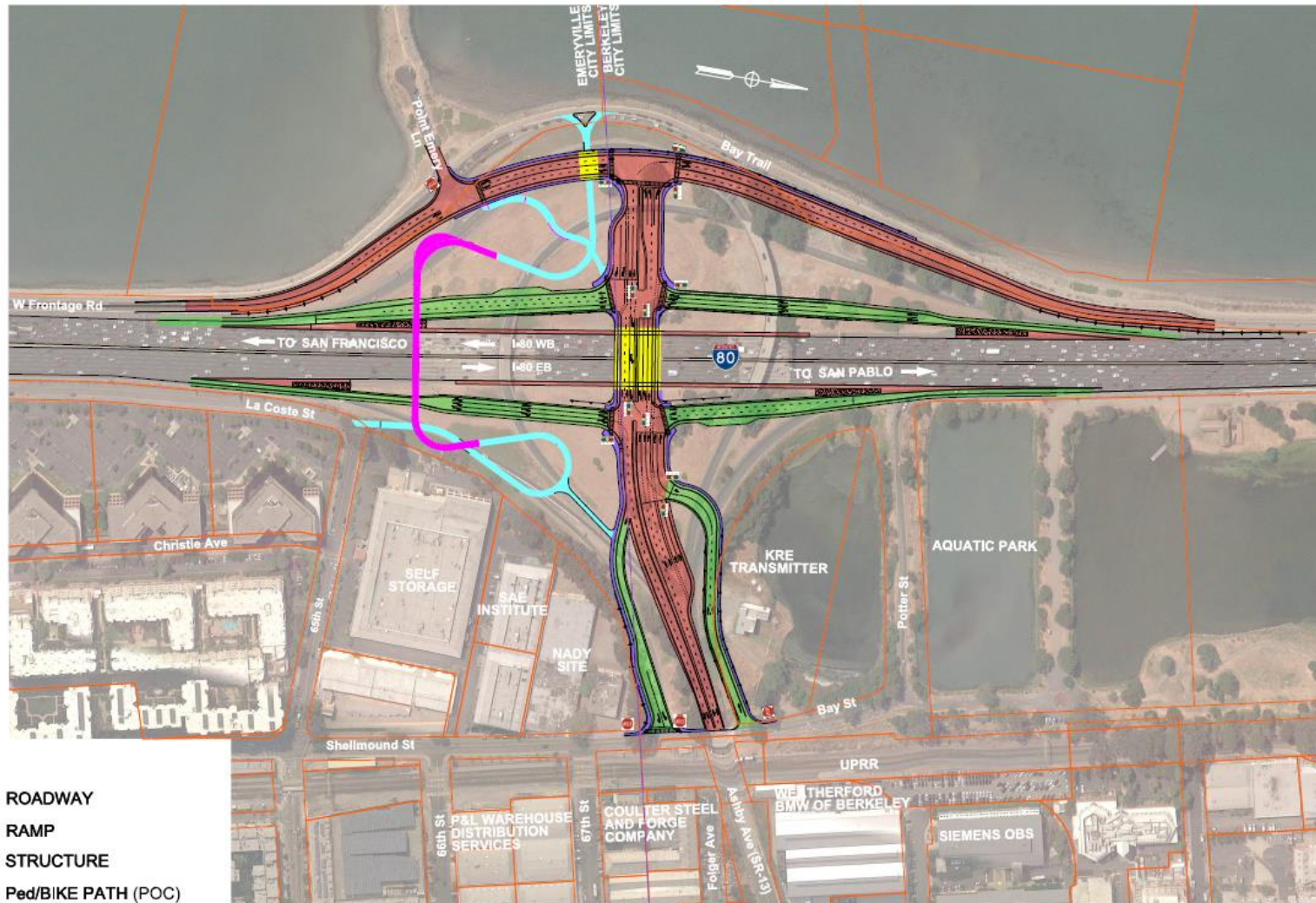
Interchange Concept Alternative - Tight Diamond Modified (T-Intersection)
