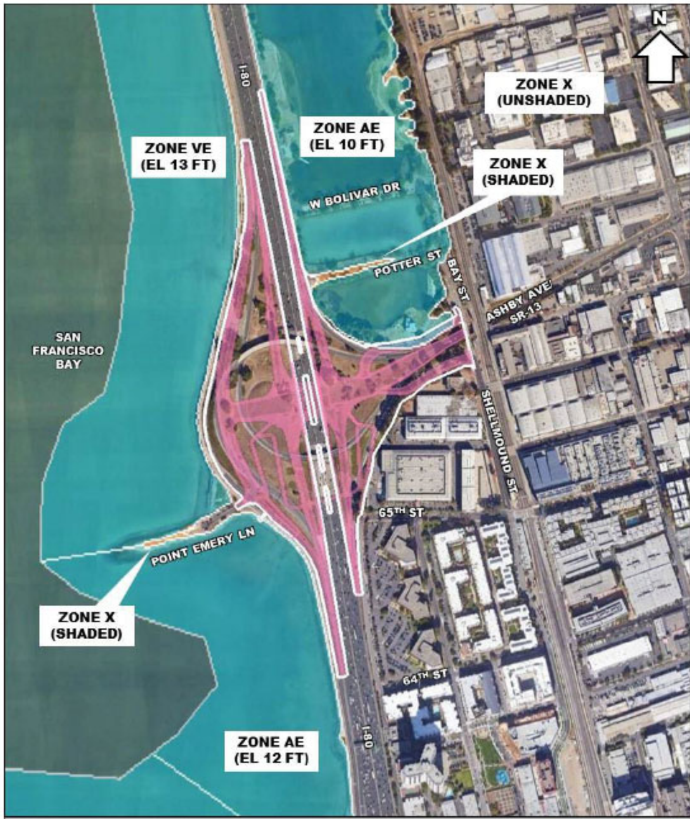
FEMA FLOODPLAIN ZONES AND BUILD ALTERNATIVE 1 (SPUI)
