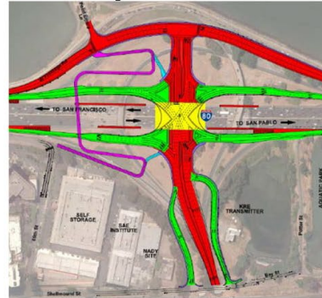
Alternative 2: Single Point Diamond with T-Intersection
