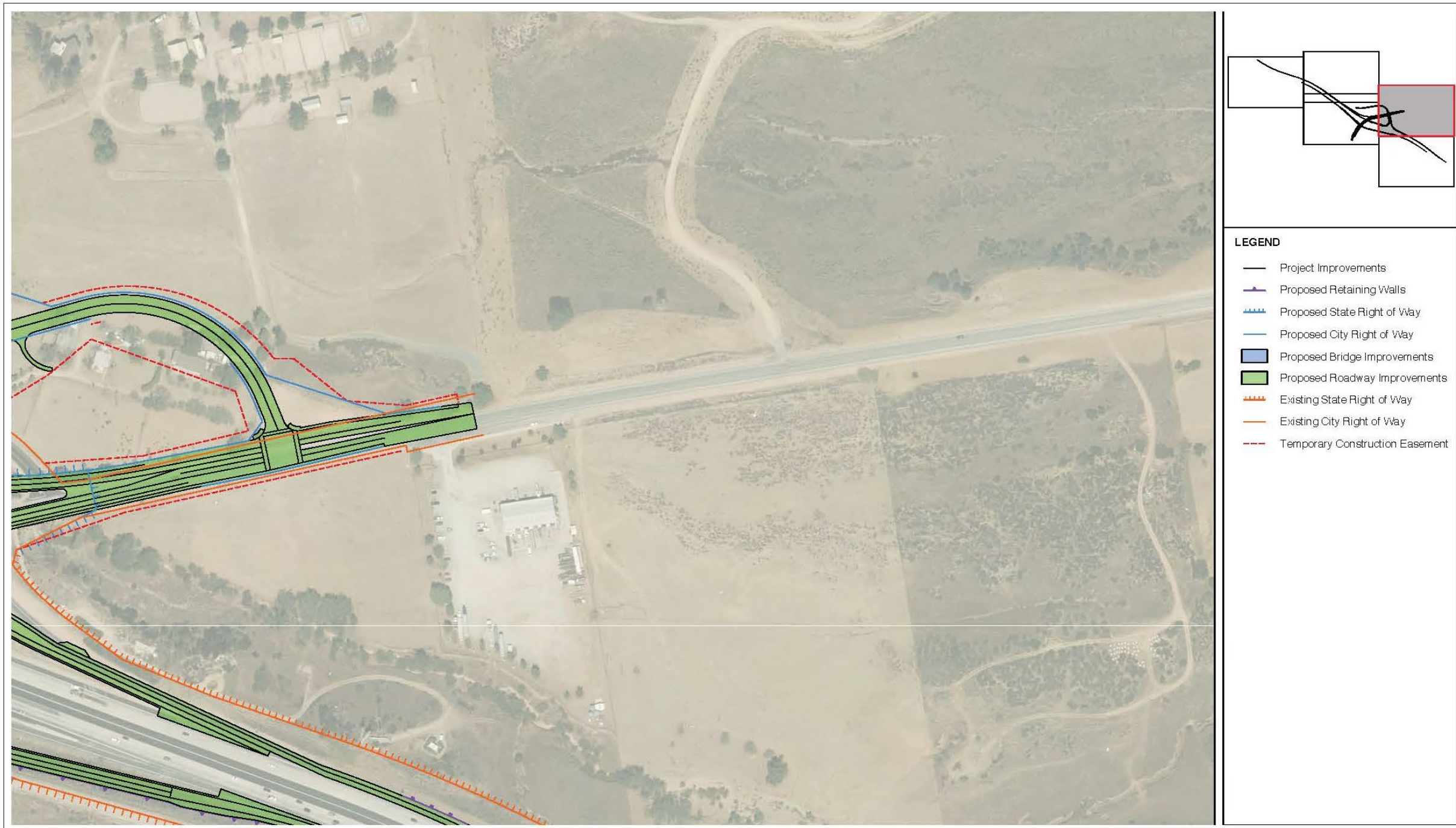
Figure 1-5d: Build Alternative 4 (Partial Cloverleaf)
