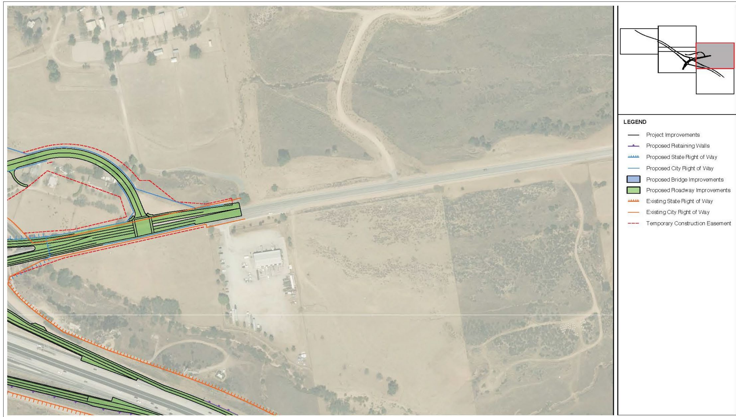
Figure 1-4d: Build Alternative 3 (Diverging Diamond)
