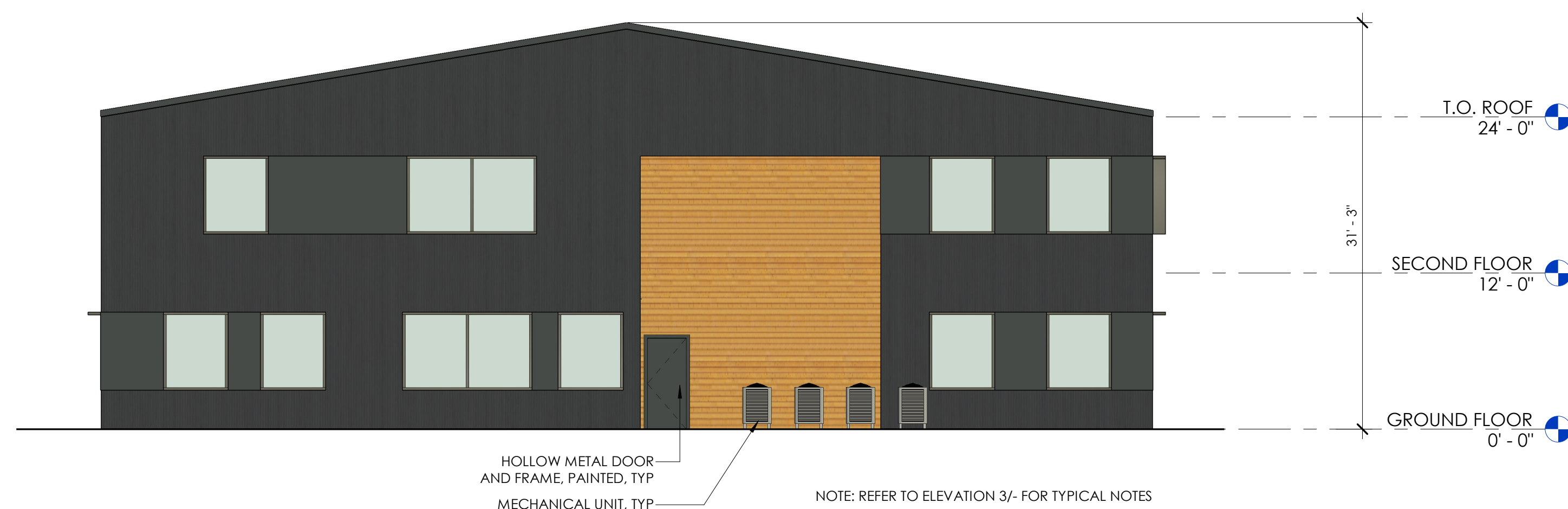
OFFICE BUILDING - NORTH ELEVATION
