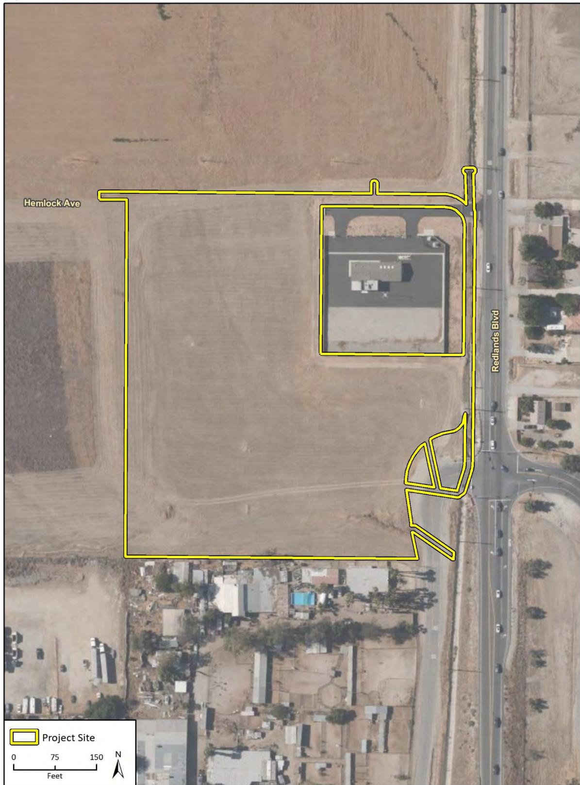
intersection of Redlands Boulevard and Hemlock Avenue, replacing the roadside drainage channel with an underground 54-inch RCP, and removal of an existing concrete box culvert that currently conveys flows under Spruce Avenue. The proposed 54-inch RCP would then outlet into an existing concrete channel south of Spruce Avenue and west of Redlands Boulevard.
