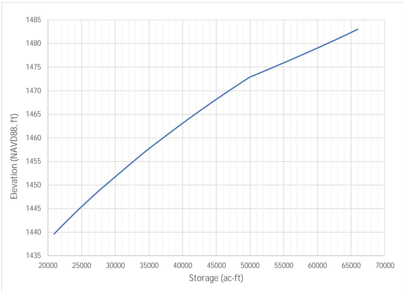
Figure 3.4. Vail Lake Elevation-Storage Curve
