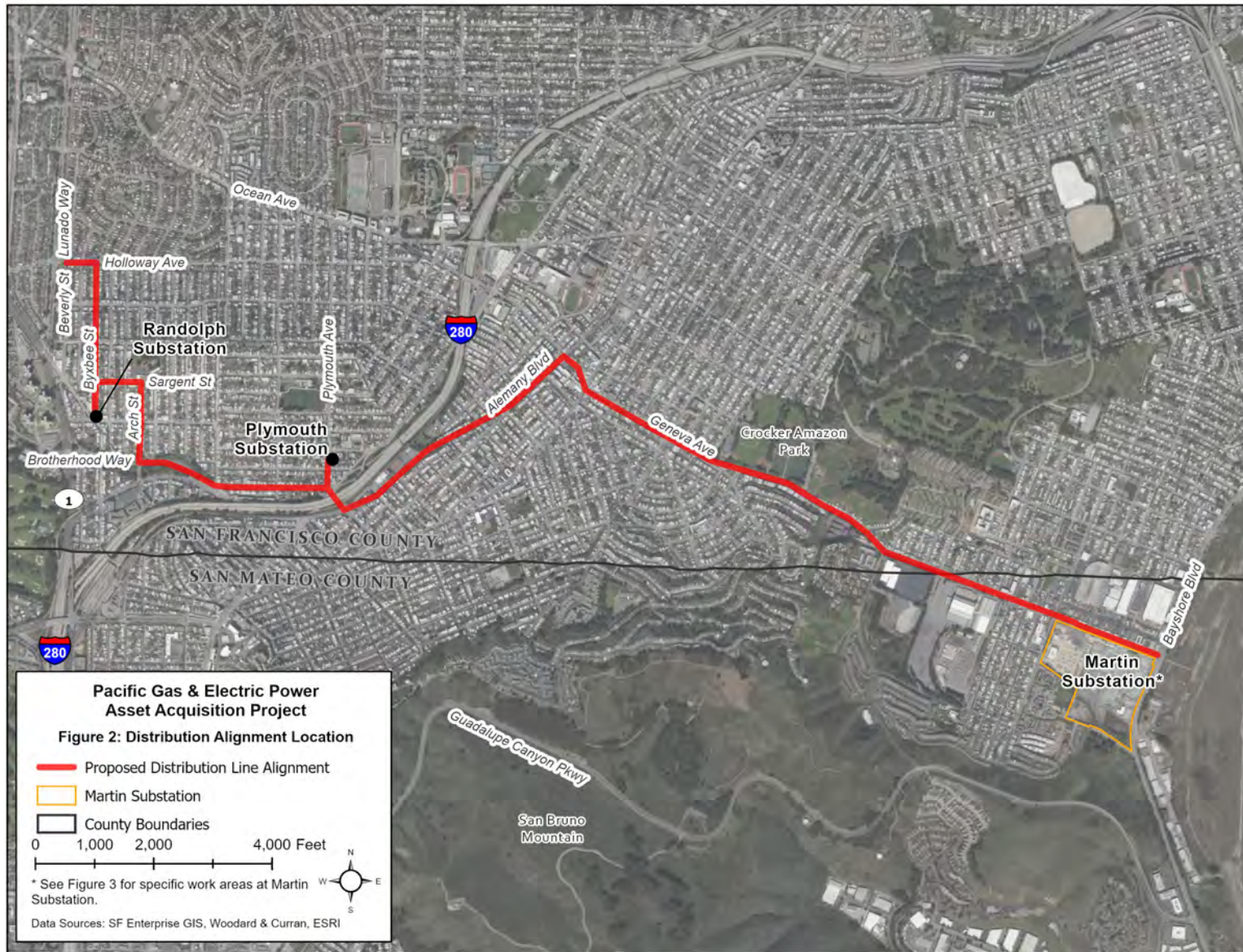
Figure 2: Distribution Alignment Location
