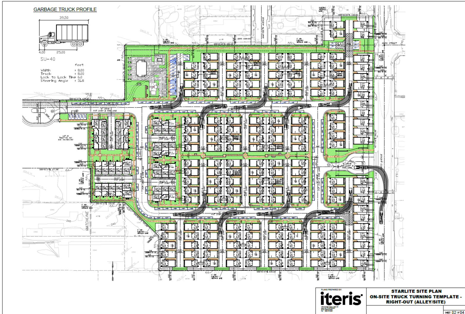
Figure 16 – Truck Turning Movements – Right Turns Out
