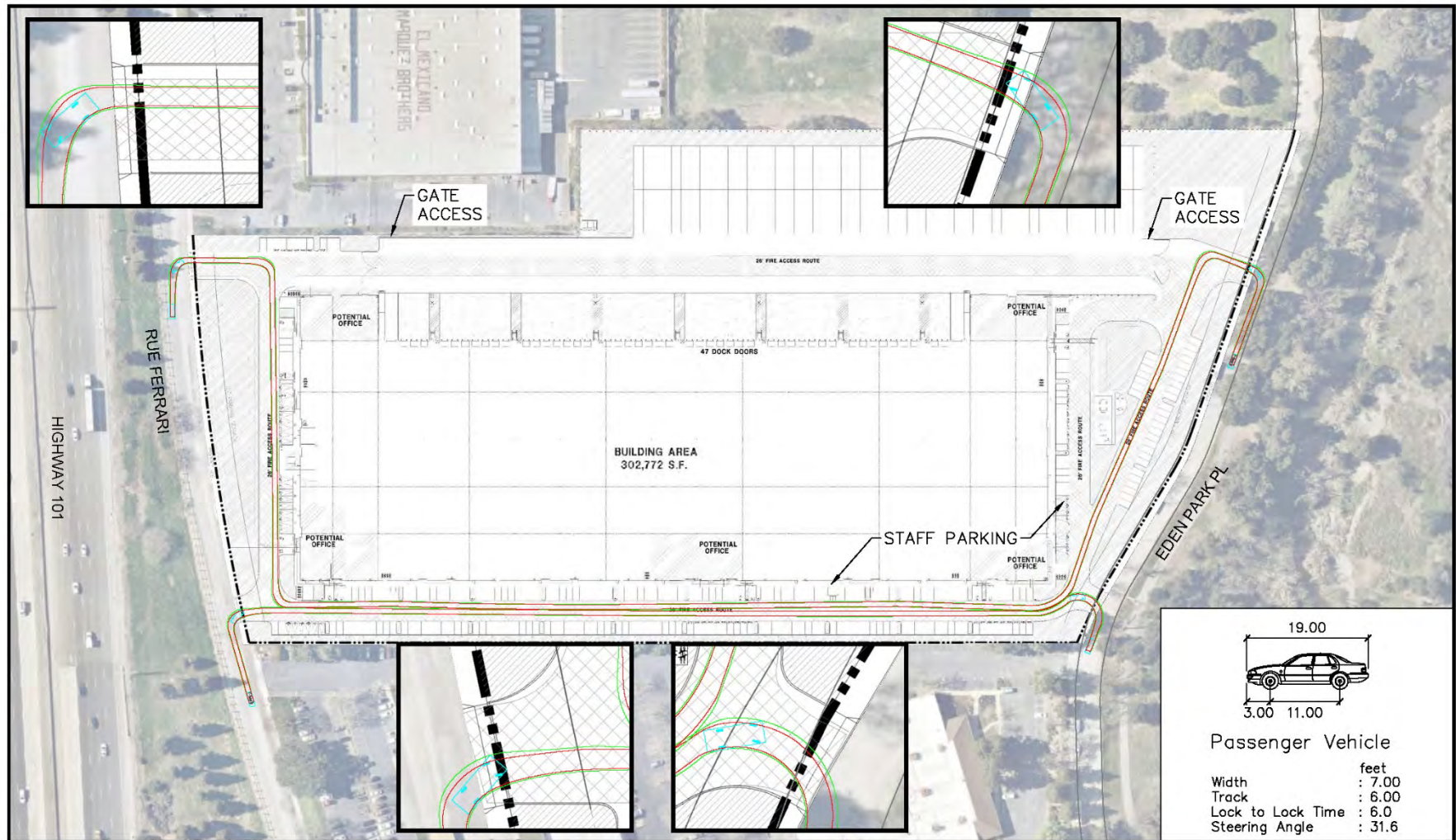
Figure 13: Passenger Vehicle Access
