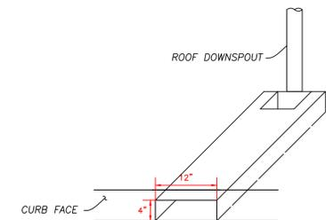
ROOF DRAIN & CURB OUTLET STRUCTURE DETAIL
