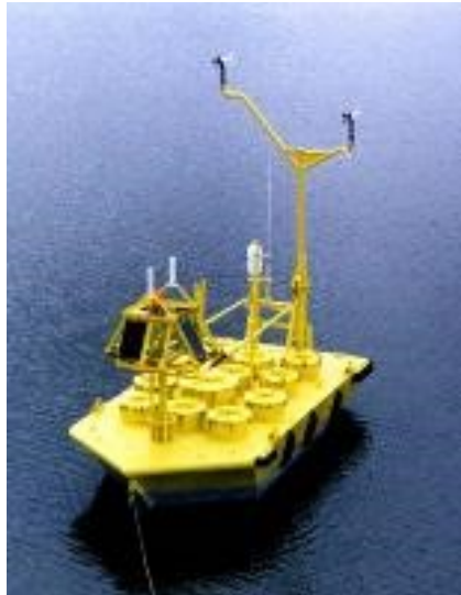
Figure 2-4: 6-Meter Boat-Shaped Hull Buoy
