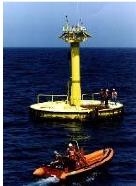
Figure 2-3: 10-Meter Discus-Shaped Hull Buoy
