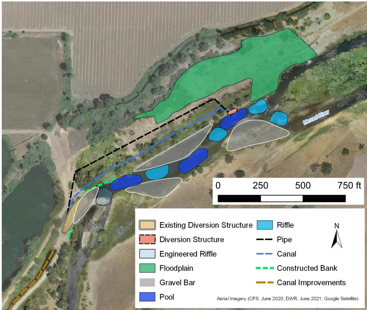
Figure 5. Conceptual design of Cowell 1 diversion enhancement.
