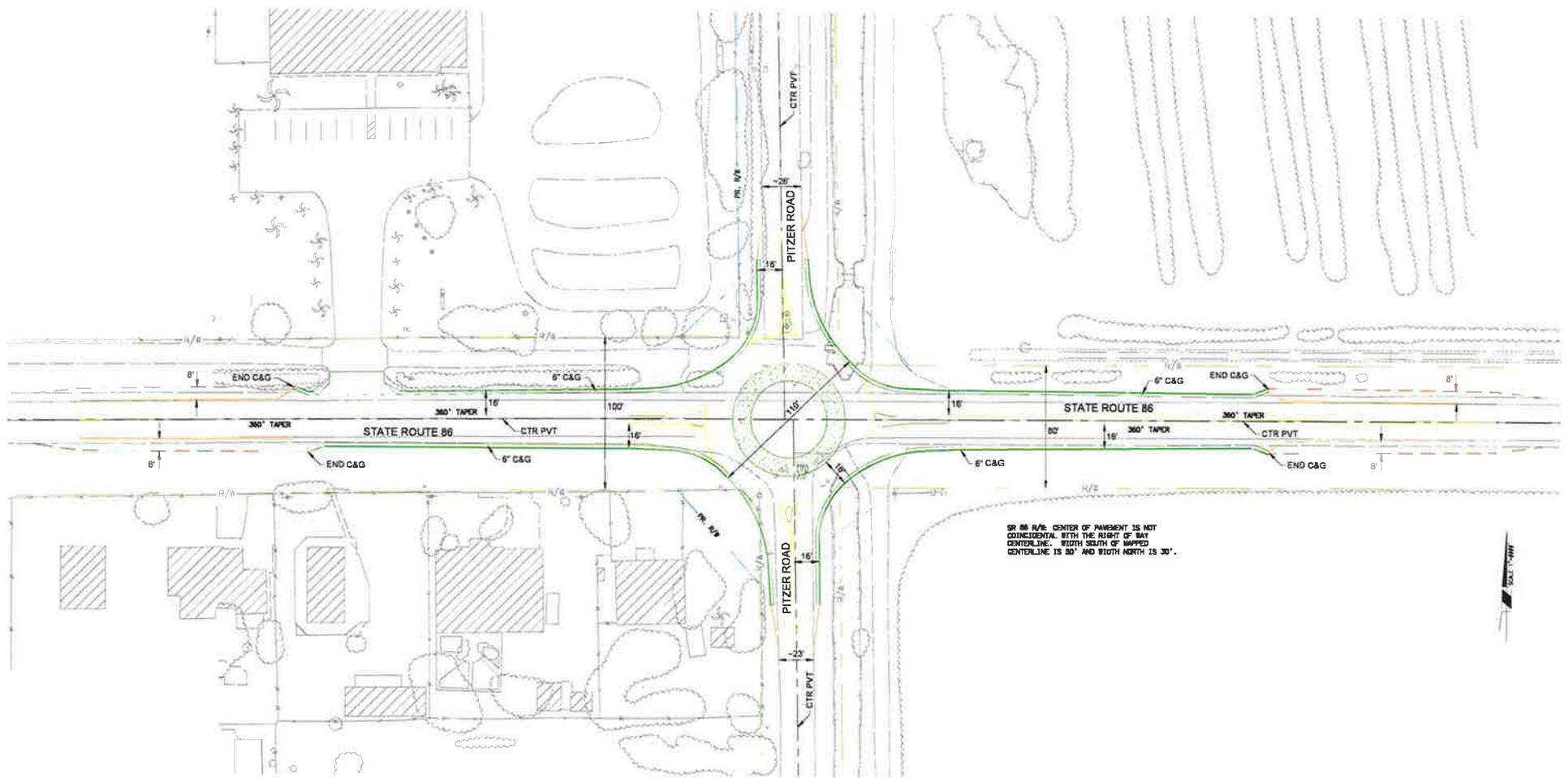
SR 86 R/W CENTER OF PAVEMENT IS NOT COINCIDENTAL WITH THE RIGHT OF WAY CENTERLINE - WITHIN SOUTH 6' MARKED CENTERLINE IS 30' AND BOTH NORTH IS 30'.
