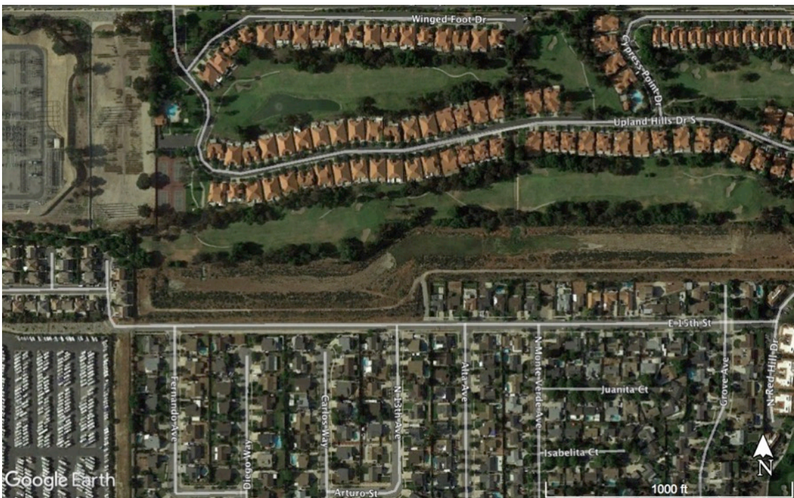
Figure 2b. May 2019 aerial photo of basin, showing vegetated slopes and floor, including green area where drain supports wetland vegetation.
