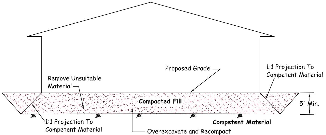
Note 1: Removal Bottom Should be Graded With Minimum 2% Fall Towards Street or Other Suitable Area (as Determined by Soils Engineer) to Avoid Ponding Below Building
