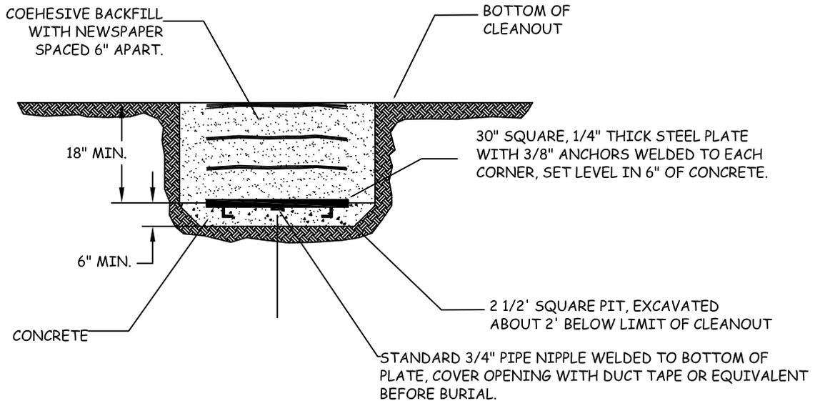
1. SURVEY FOR HORIZONTAL AND VERTICAL LOCATION TO NEAREST .01 INCH PRIOR TO BACKFILL USING KNOW LOCATIONS THAT WILL REMAIN INTACT DURING THE DURATION OF THE MONITORING PROGRAM. KNOW POINTS EXPLICITLY NOT ALLOWED ARE THOSE LOCATED ON FILL OR THAT WILL BE DESTROYED DURING GRADING.
