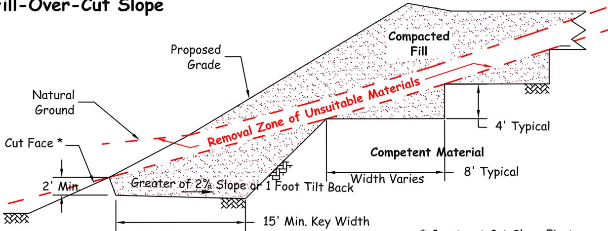
\* Construct Cut Slope First
