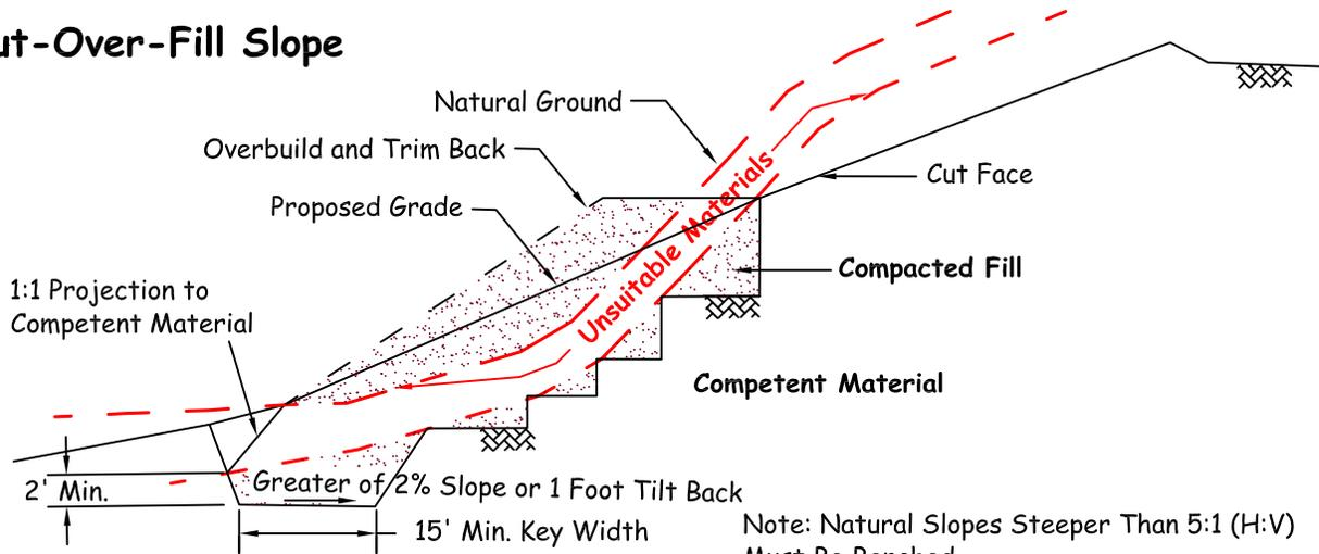
Note: Natural Slopes Steeper Than 5:1 (H:V) Must Be Benched.
