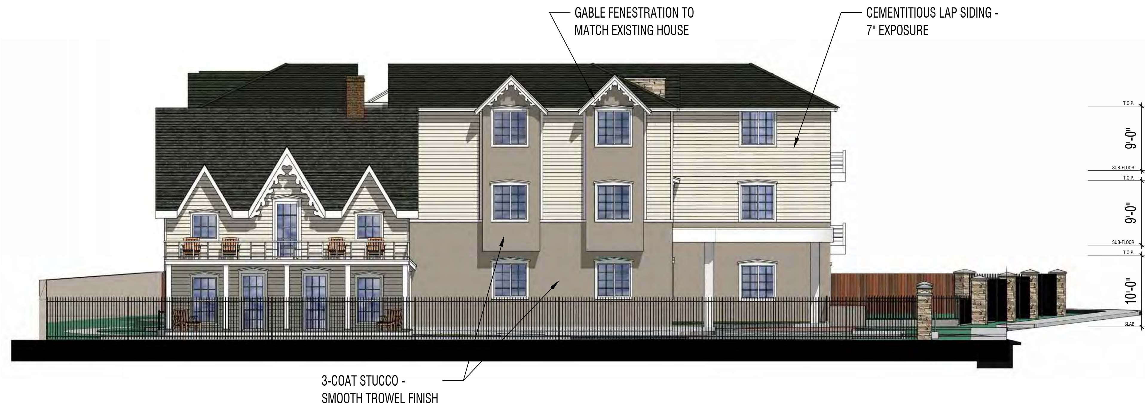
EAST ELEVATION (LEFT SIDE)
