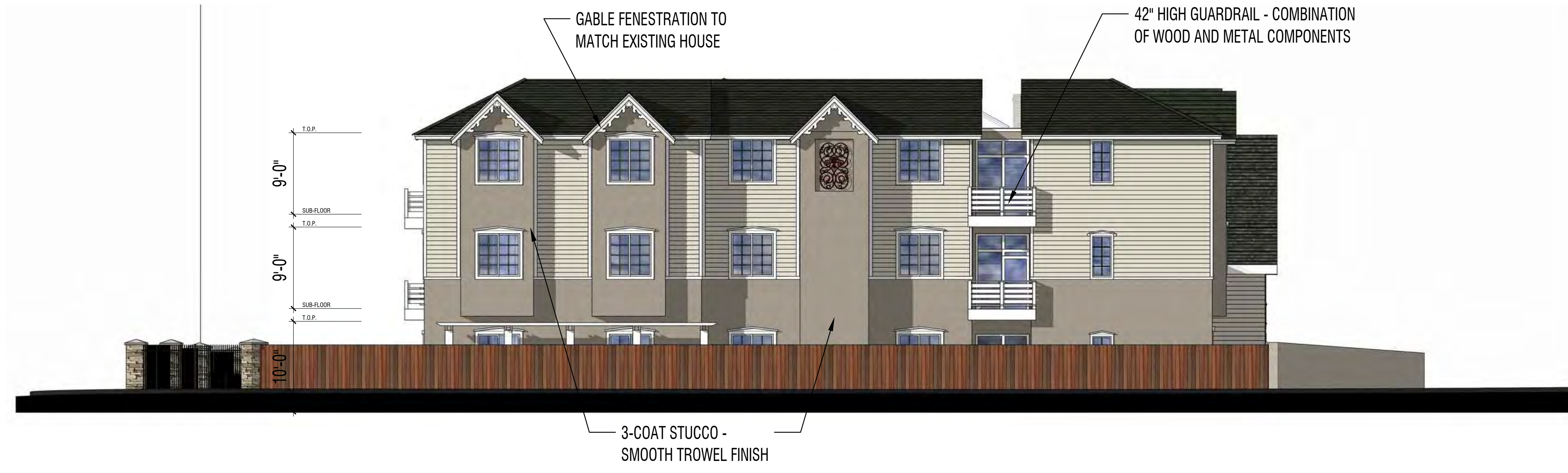
WEST ELEVATION (RIGHT SIDE)
