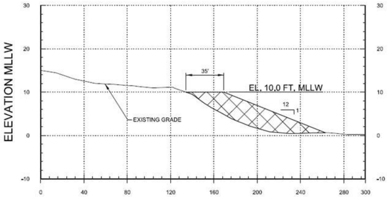
**Figure 8. Newport Beach Sand Backpass Fill Cross Section**
