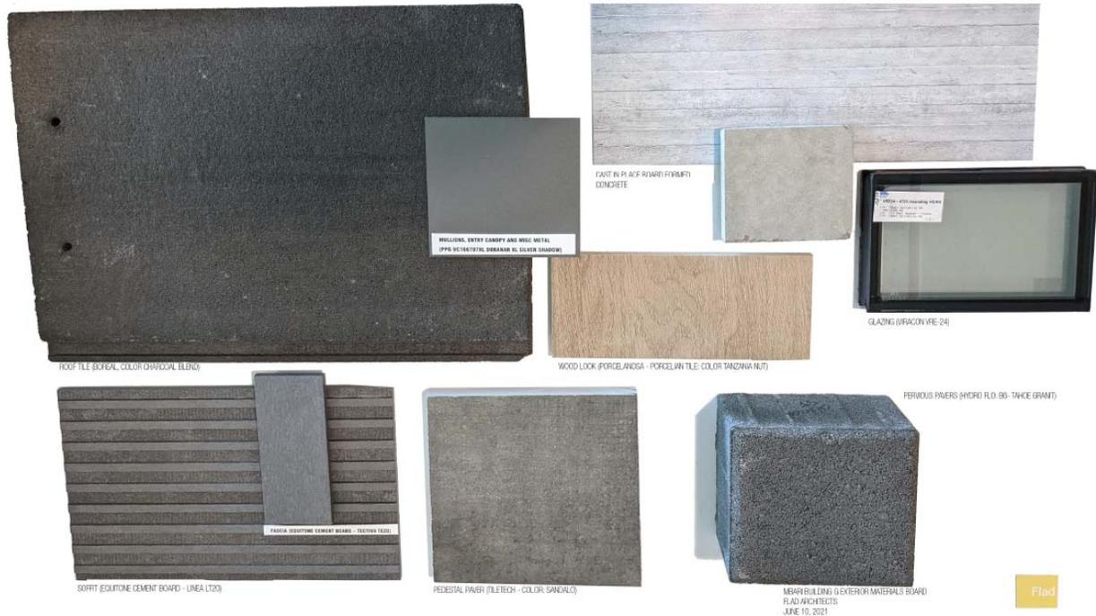
*Exhibit 14: Photo of material sample board for the project. From left to right, finish materials include: charcoal grey roof tiles, grey mullions, wood look porcelain tiles, cast in place concrete (board formed and smooth), glass glazing, cement board soffits, and grey pedestrian pavers. (Source IX.1)*
