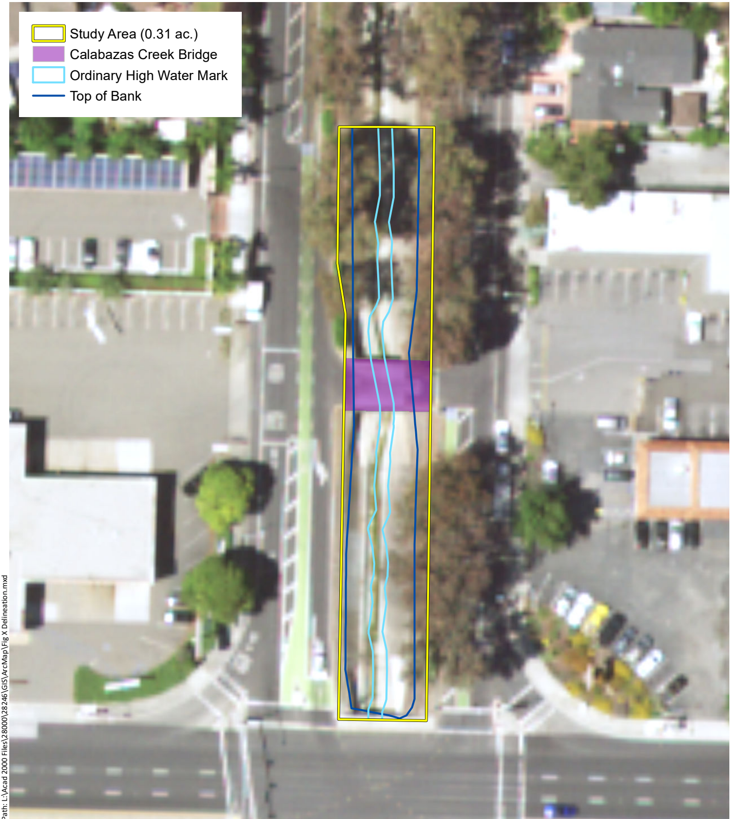
Figure 1. Top of Bank and Ordinary High Water Mark
