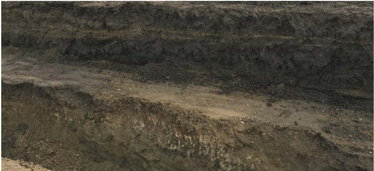
Figure 8. SE wall of Trench T-1 showing artificial fill layers over the natural soil. Note the abundant calcite concentrations underlying the black ABb horizon.
