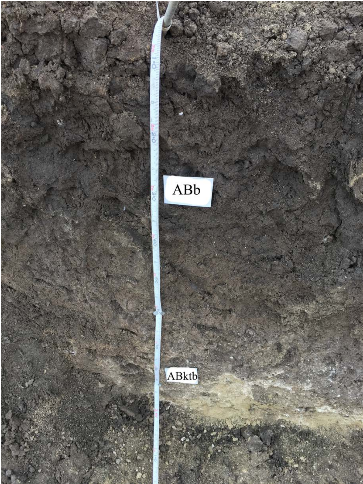
Figure 2. Lower portion of the ABb horizon overlying the ABktb horizon of Soil Profile No. 1.
