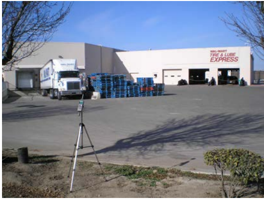
Truck Loading/Unloading Noise Measurement
