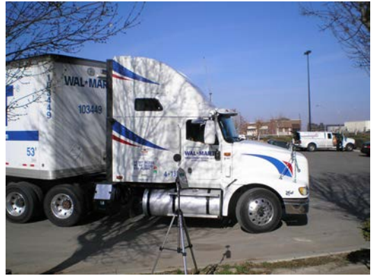
Truck Loading/Unloading Noise Measurement
