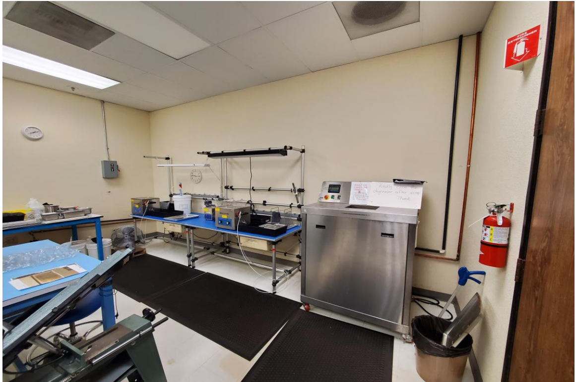
Photograph No. 7: Self-contained degreaser in Silitronics equipment maintenance room.
