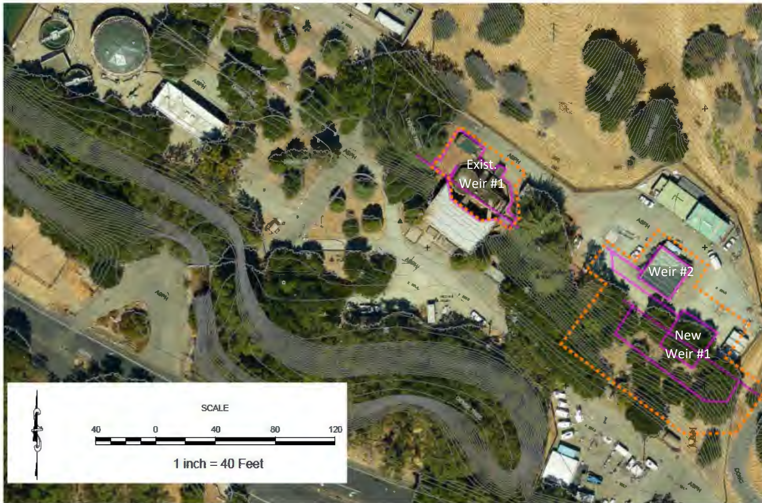
Figure 4: Lafayette WTP Conceptual Site Plan
