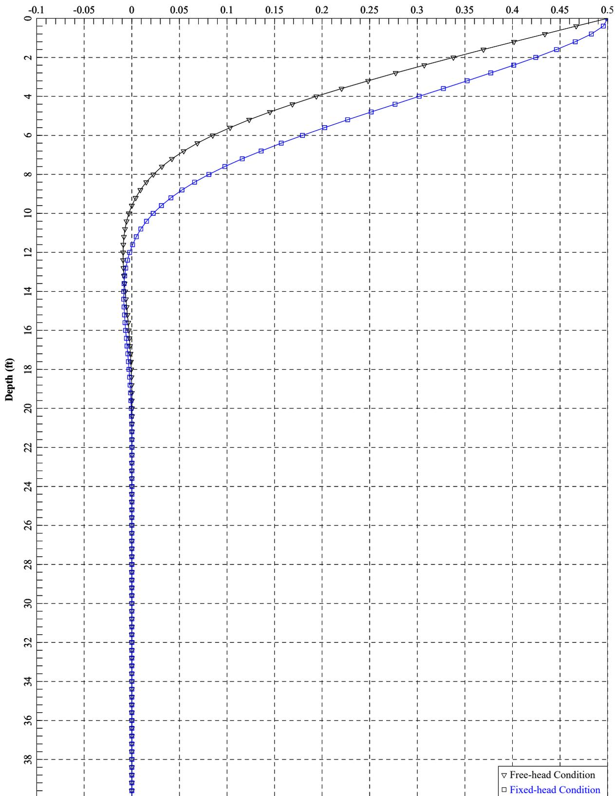
18-inch-diameter ACIP/APGD Pile (Static)
