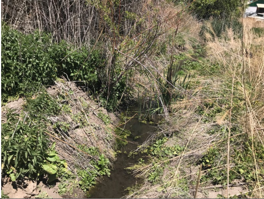
Photograph 13: (32.691758, 116.339728) East-facing view of the 4-foot wide earthen bottom channel on the central portion of the project site. This photo shows where sampling point NW-11 was taken to determine the presence of OHWM indicators.
