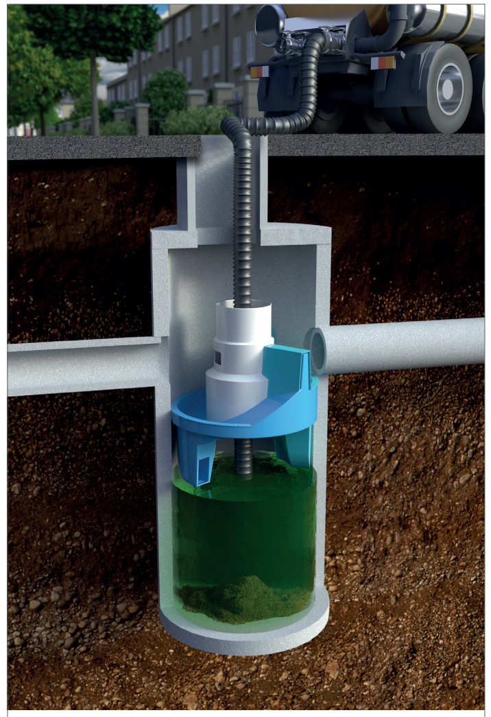
Fig.4 Floatables are removed with a vactor hose
