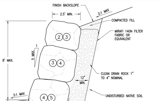
UNLESS OTHERWISE SPECIFIED IN WRITING BY THE ROCKERY "DESIGNER," ALL ROCKS PLACED ON LOWER ONE-THIRD TO ONE-HALF OF THE WALL SHALL BE 2000 LBS OR LARGER. ROCKS PLACED ABOVE THIS LEVEL SHALL GRADUALLY DECREASE IN SIZE WITH INCREASING WALL HEIGHT.
