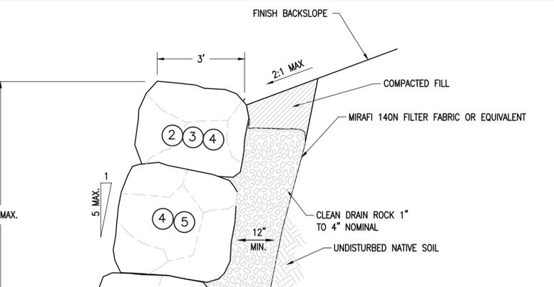
UNLESS OTHERWISE SPECIFIED IN WRITING BY THE ROCKERY "DESIGNER," ALL ROCKS PLACED ON LOWER ONE-THIRD TO ONE-HALF OF THE WALL SHALL BE 2000 LBS OR LARGER. ROCKS PLACED ABOVE THIS LEVEL SHALL GRADUALLY DECREASE IN SIZE WITH INCREASING WALL HEIGHT.
