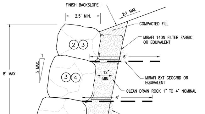
UNLESS OTHERWISE SPECIFIED IN WRITING BY THE ROCKERY "DESIGNER," ALL ROCKS PLACED ON LOWER ONE-THIRD TO ONE-HALF OF THE WALL SHALL BE 2000 LBS OR LARGER. ROCKS PLACED ABOVE THIS LEVEL SHALL GRADUALLY DECREASE IN SIZE WITH INCREASING WALL HEIGHT.
