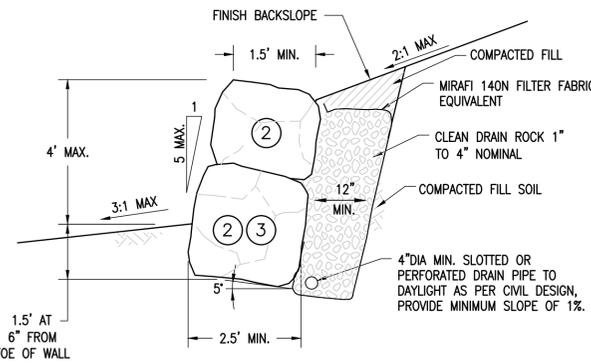
UNLESS OTHERWISE SPECIFIED IN WRITING BY THE ROCKERY "DESIGNER," ALL ROCKS PLACED ON LOWER ONE-THIRD TO ONE-HALF OF THE WALL SHALL BE 700 LBS OR LARGER. ROCKS PLACED ABOVE THIS LEVEL SHALL GRADUALLY DECREASE IN SIZE WITH INCREASING WALL HEIGHT.
