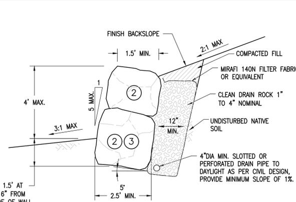
UNLESS OTHERWISE SPECIFIED IN WRITING BY THE ROCKERY "DESIGNER," ALL ROCKS PLACED ON LOWER ONE-THIRD TO ONE-HALF OF THE WALL SHALL BE 700 LBS OR LARGER. ROCKS PLACED ABOVE THIS LEVEL SHALL GRADUALLY DECREASE IN SIZE WITH INCREASING WALL HEIGHT.
