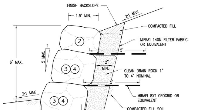
UNLESS OTHERWISE SPECIFIED IN WRITING BY THE ROCKERY "DESIGNER," ALL ROCKS PLACED ON LOWER ONE-THIRD TO ONE-HALF OF THE WALL SHALL BE 700 LBS OR LARGER. ROCKS PLACED ABOVE THIS LEVEL SHALL GRADUALLY DECREASE IN SIZE WITH INCREASING WALL HEIGHT.
