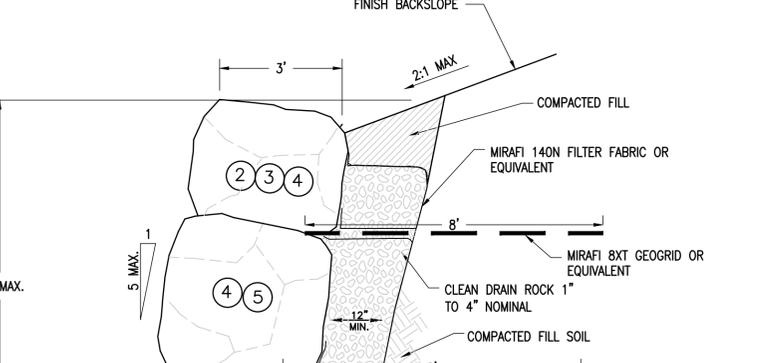
UNLESS OTHERWISE SPECIFIED IN WRITING BY THE ROCKERY "DESIGNER," ALL ROCKS PLACED ON LOWER ONE-THIRD TO ONE-HALF OF THE WALL SHALL BE 2000 LBS OR LARGER. ROCKS PLACED ABOVE THIS LEVEL SHALL GRADUALLY DECREASE IN SIZE WITH INCREASING WALL HEIGHT.
