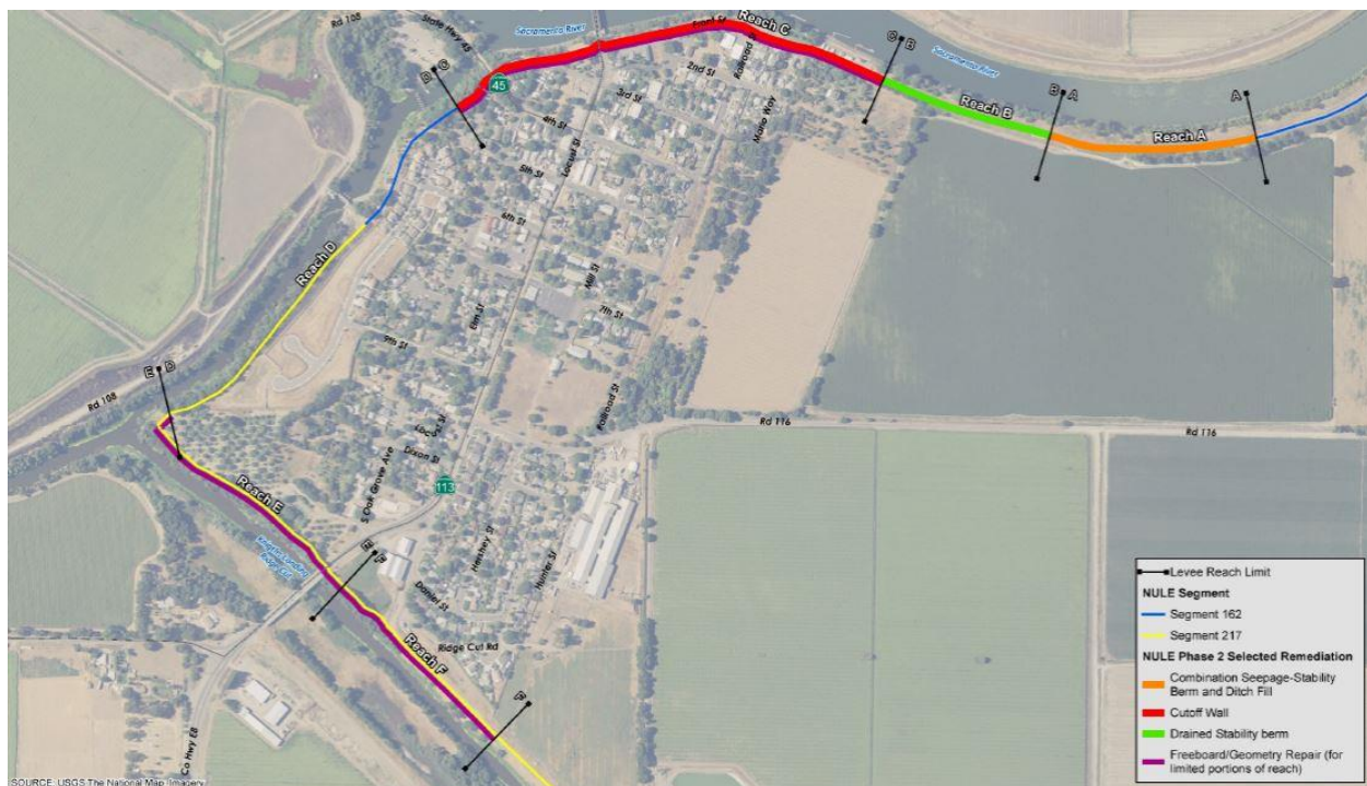
Figure 1. Seepage Concerns Along Sacramento River State Plan of Flood Control Levee
