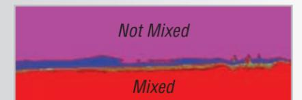
Stratified tank due to single inlet pipe.
