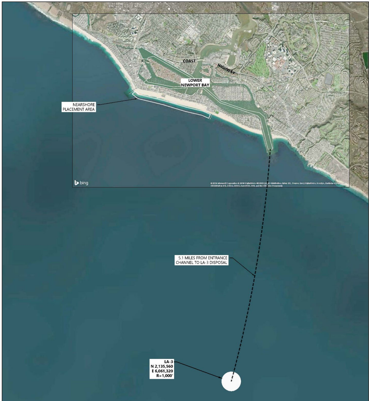
Figure 1. Overview of project area, showing the Lower Newport Harbor Bay channels, proposed nearshore disposal site along the beach, and ocean disposal site LA-3.
