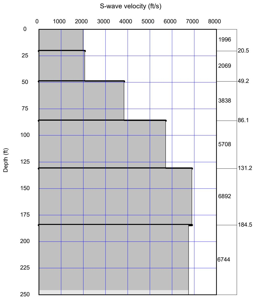
**SHEAR-WAVE VELOCITY MODEL: Average Vs 100ft = 2,763.8 ft/sec**
