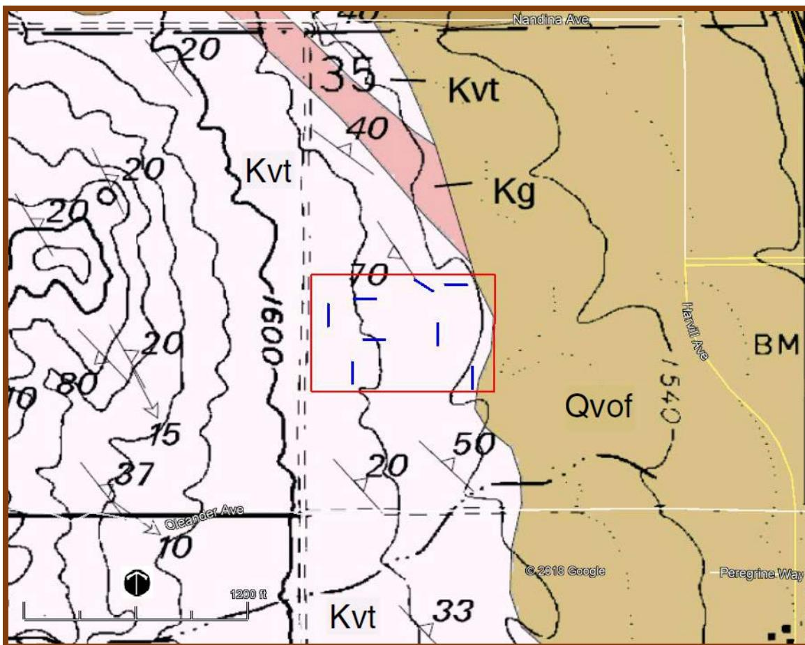
**FIGURE 1- Geologic Map (Morton, 2003), Seismic traverses shown as blue lines.**
