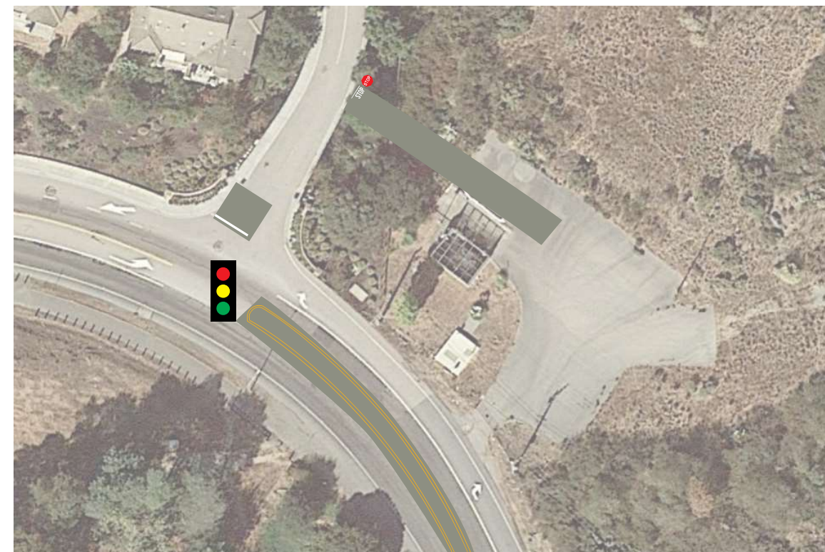
Access Alternative 4: Traffic Signal at the Intersection of Sir Francis Drake Boulevard and Drakes Cove Road, Acceleration Lane Changed to Painted Median on Sir Francis Drake Boulevard, and Internal Access Road to Drakes Cove Road.
