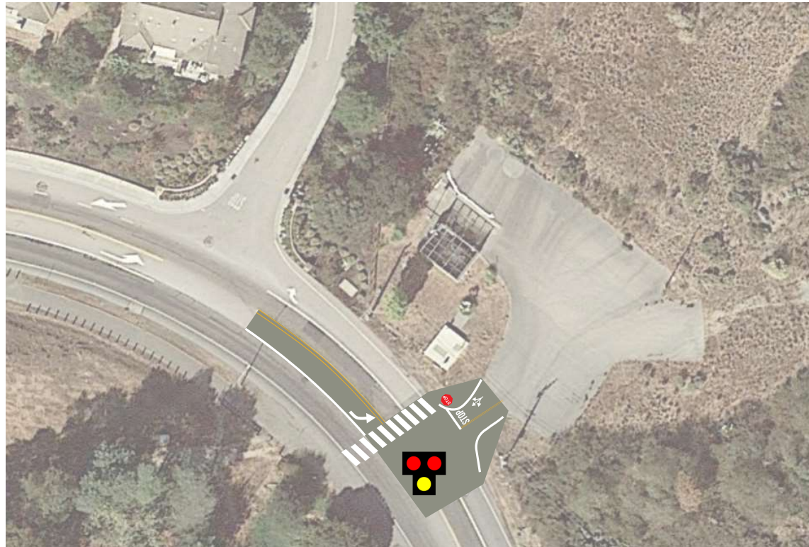
Access Alternative 1: Stop Sign at Project Driveway, Acceleration Lane Changed to Left-Turn Lane on Sir Francis Drake Boulevard, and Crosswalk from Project Driveway to the Class I Multi-use Path with HAWK Beacon.
