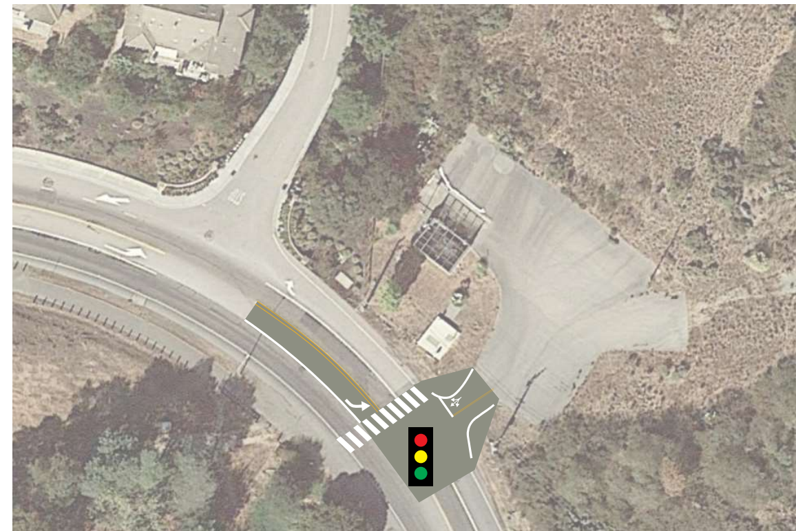
Access Alternative 2: Traffic Signal at Project Driveway, Acceleration Lane Changed to Left-Turn Lane on Sir Francis Drake Boulevard, and Crosswalk from Project Driveway to the Class I Multi-use Path.
