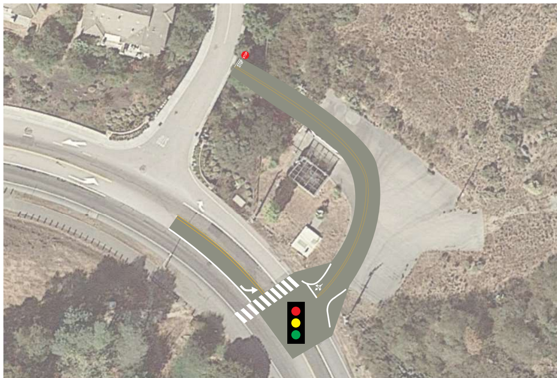
Access Alternative 3: Traffic Signal at Project Driveway, Acceleration Lane Changed to Left-Turn Lane on Sir Francis Drake Boulevard, Crosswalk from Project Driveway to Class I Multi-use Path, and Internal Access Road to Drakes Cove Road.
