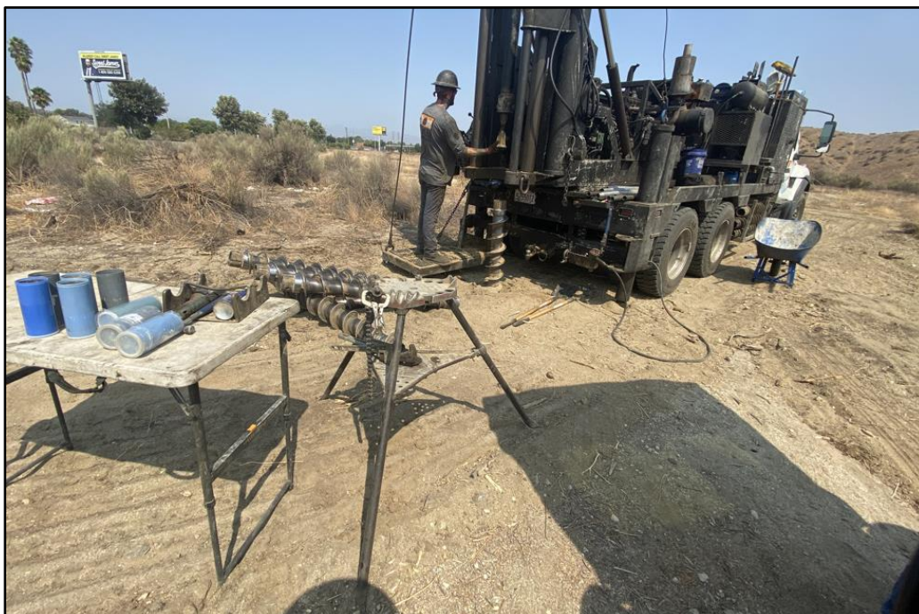
Figure 24. View of geologic boring conducted in the middle southern area of the Project site
