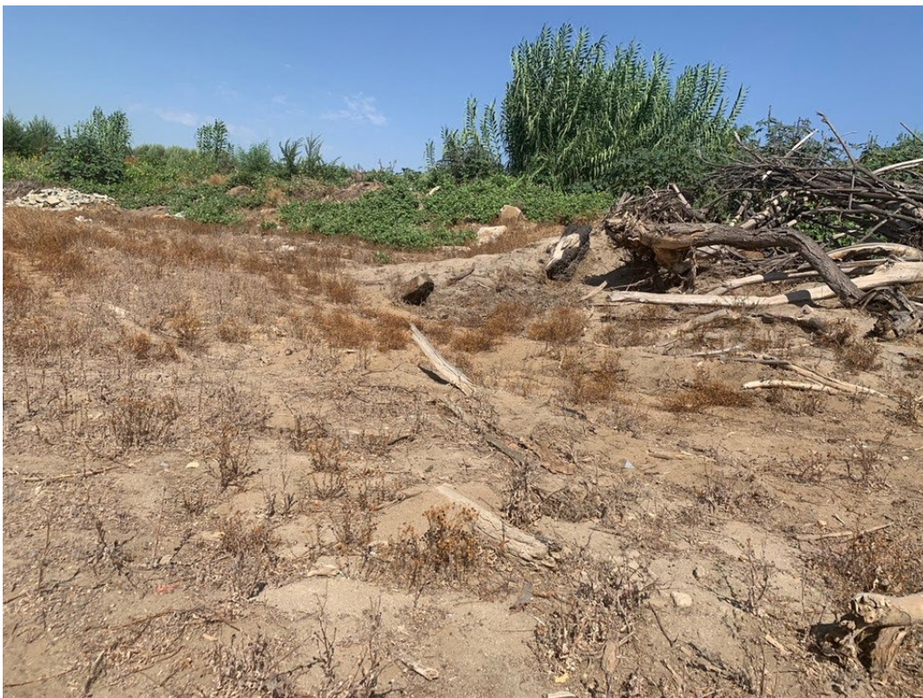
Photograph 4: The Delhi Sand soils on the south side of the Jurupa Ditch are heavily contaminated with clay from the surrounding soils and from infiltration of silts and fines from river water flowing through the middle of the soils over the last 140 years.
