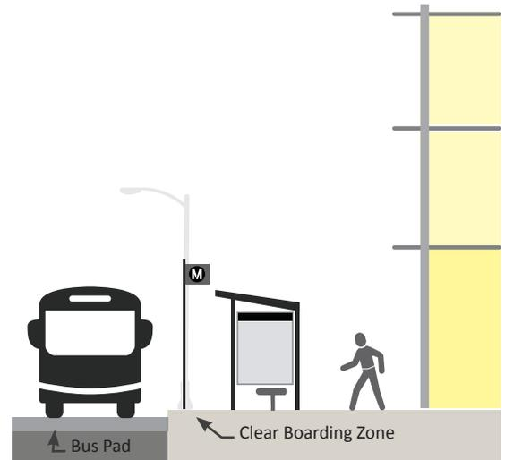
*A concrete bus pad should be located at bus stops and bus shelters should be located along sidewalks to ensure an accessible path of travel to a clear boarding area.*
