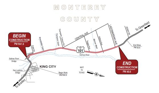
Culvert work would occur at post miles 43.65, 45.17, and 47.68. Two linear ditches along the westerly right-of-way would be filled in and regraded. Rock slope protection or concrete ditch lining will likely be needed to reduce the potential for scour and sediment transport. The pavement at the weigh-in-motion station at post mile 48.0 in Greenfield will be reconstructed and lengthened to 300 feet.
