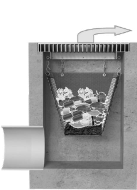
1. Remove grate and set up vacuum truck to clean the filter basket.
