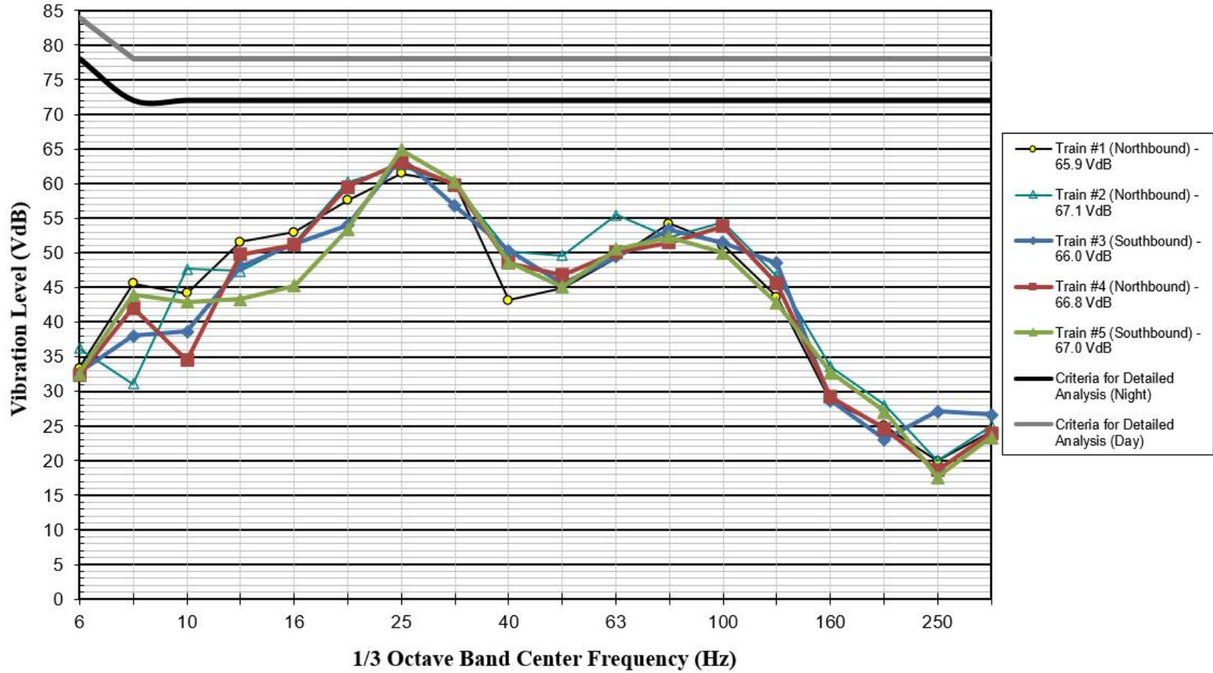
**FIGURE A8 VTA Light Rail Train Vibration Levels at V-2**
