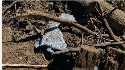
**Figure 4.** This is a view of an ingot or solidified molten metal, possibly resulting from the recent fire. Low melting point and sheen, as well as weight, suggest it may be lead or other similar metal .
