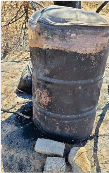
**Figure 7.** This is a view of a distorted 50-gallon drum with leakage at the bottom as evidenced by the stained soil.
