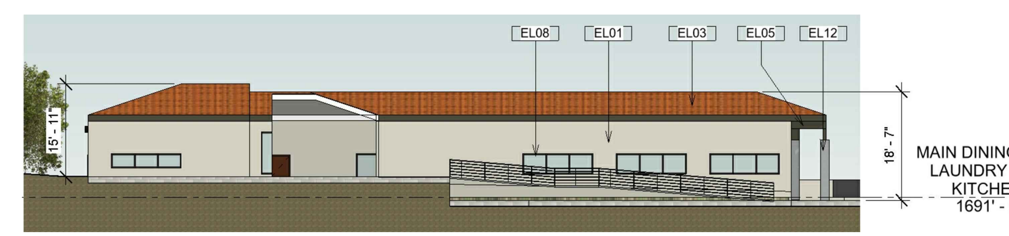
4 BLDG 6 DINING HALL EAST ELEVATION SCALE: 1/16" = 1'-0"
