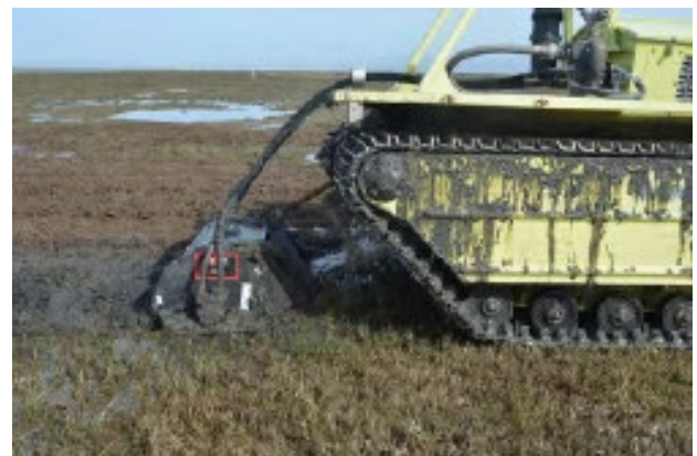
Image 2-1 – Representative Vegetation Removal Equipment. Handheld brushcutter/grinding method (left) used to remove above-ground vegetation. Marshmaster (right) used to mow larger areas and grind (via rototiller) dense-flowered cordgrass rhizomes. Photo credit: A. Pickart (USFWS 2017).
