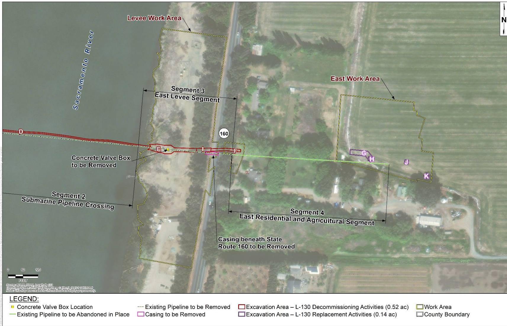
Figure 2-15. Decommissioning Project Overview (East)
