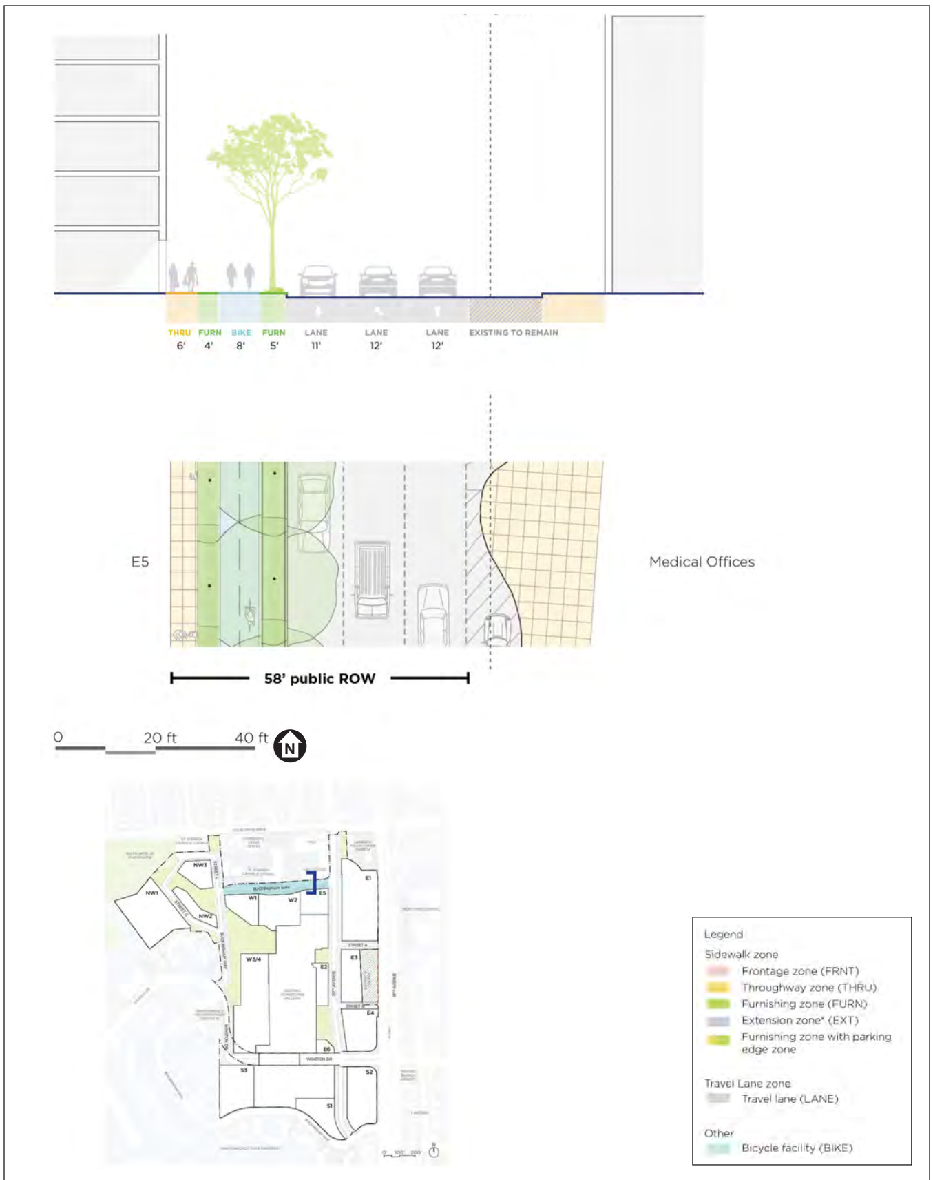
FIGURE 2-18 BUCKINGHAM WAY NORTH ILLUSTRATIVE SECTION (REVISED) 2-12
