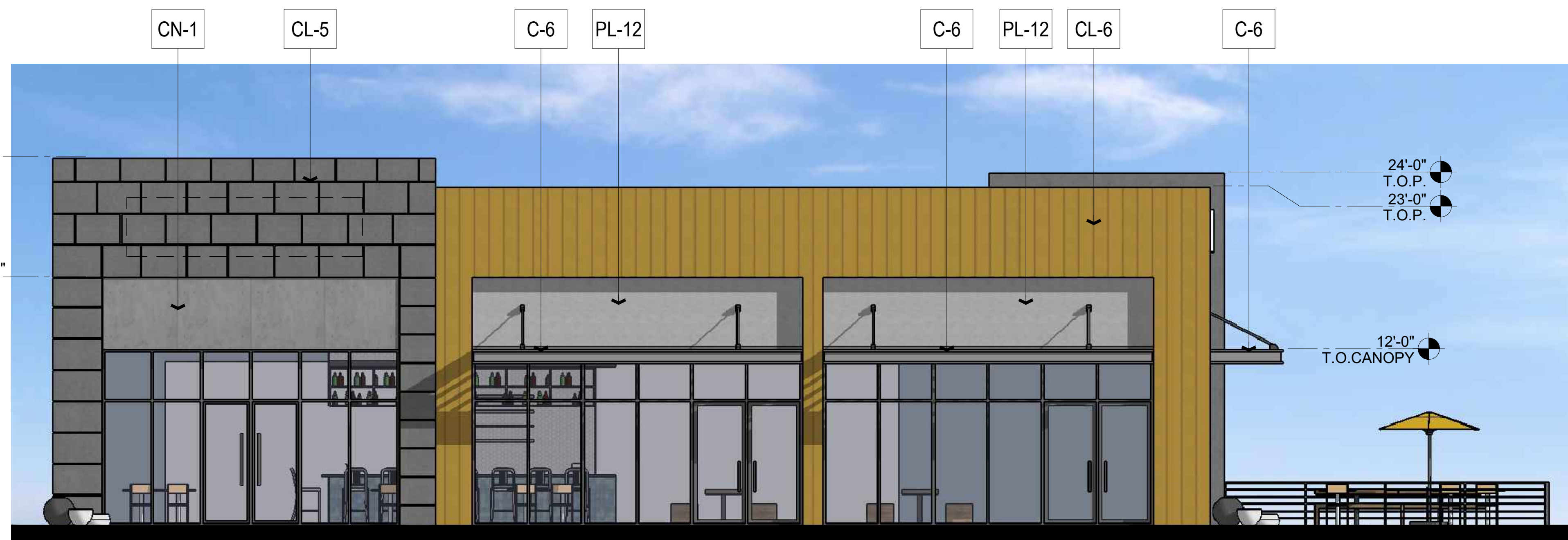
W EXTERIOR ELEVATION- WEST 3/16" = 1'-0"
