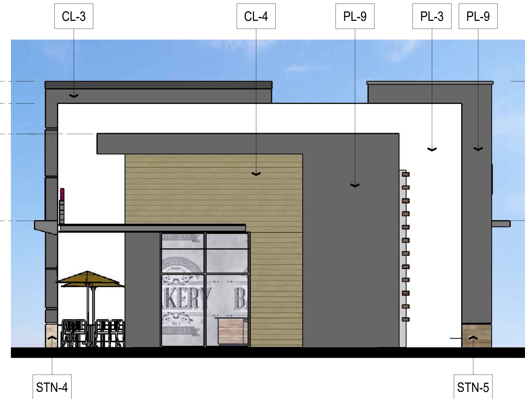
N EXTERIOR ELEVATION- NORTH 3/16" = 1'-0"
